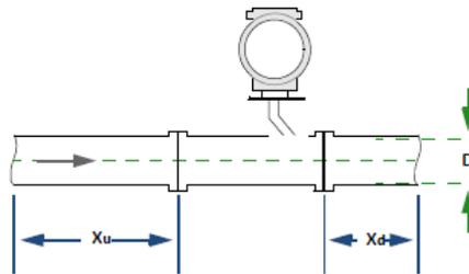
Image 5. Installation of In-line Meters (representative)
