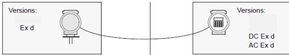
**Image 2. Transmitter Separate Configuration**
