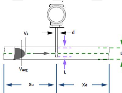
**Image 4. Installation of Insertion Meters (representative)**
